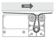
Unscrew plate [A] and insert the belt as shown in figure. Close the plate and tighten the screws.
